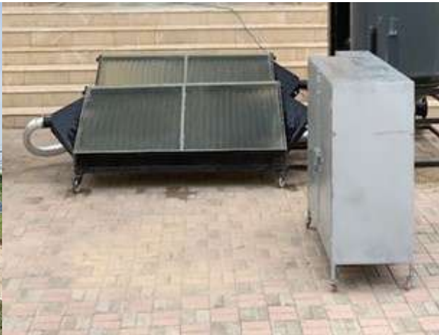
A SOLAR DESICCANT CABINET DRYER FOR FRUITS
