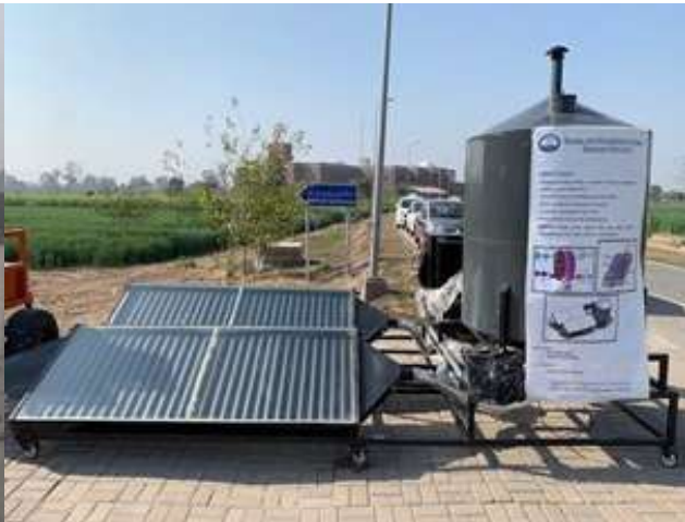
SOLAR DESICCANT DRYER FOR GRAINS
